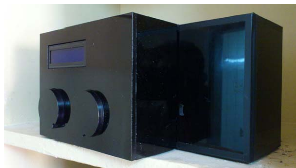
Figure 3. Instrument for producing an alternating magnetic field (MG12). [Color figure can be viewed in the online issue, which is available at wileyonlinelibrary.com .]
